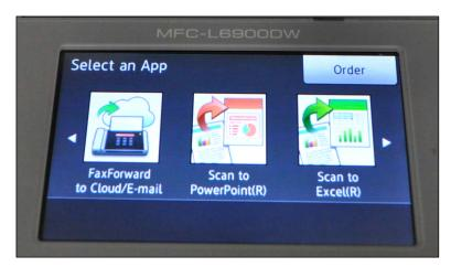
Web Connect also includes standard OCR capabilities, letting users scan to searchable PDF and editable MS Office files right at the panel, eliminating the need for additional processing back at the PC.
